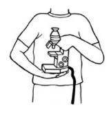
2. Carefully remove the scope from the cabinet by gripping the *arm of microscope* by one hand and holding the *base of the microscope* with the other hand. Always carry the microscope with both hands.
